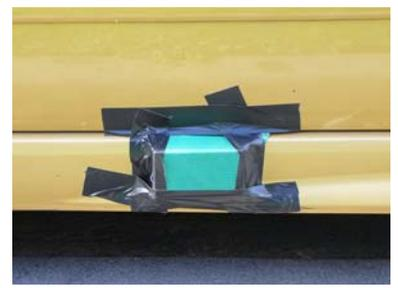
Remember the Dorian transmitter must remain in the direction of vehicle travel, ie **FRONT to BACK** on the vehicle, and **not across the vehicle nor vertical on the vehicle**. Please do not place it near the exhaust outlet as this can melt the bag and allow the Dorian transmitter to fall out and be damaged. **Lost and/or damaged Dorian transmitters will be charged to the you, the hirer at \$250.00 each.**
