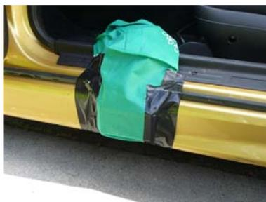
Close the car door on the excess bag and tape the Dorian transmitter bag securely to the car sill
