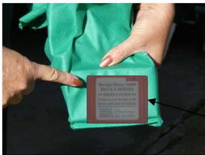
Then fold the bag so the Dorian transmitter is flat and the excess bag is laying behind it. Check the orientation of the Dorian transmitter, it must be installed with the longest side running from front to back of the vehicle
