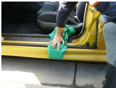
Open the door of the vehicle and place all the excess bag in the door opening and tape the Dorian transmitter to the door sill securing the bag so that it can not fall out of the car
